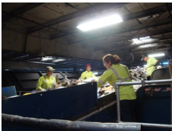
Casella employees pre-sort out material that may damage equipment, like plastic bags and large metal objects.
